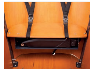
Battery underneath the bench
